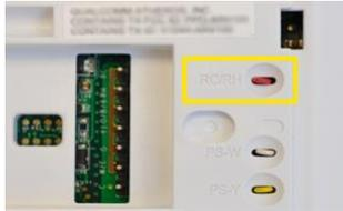
Clip the jumper on the back of the thermostat
