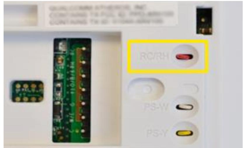
No jumpers are required when installing the Sensi Wi-Fi Thermostat
